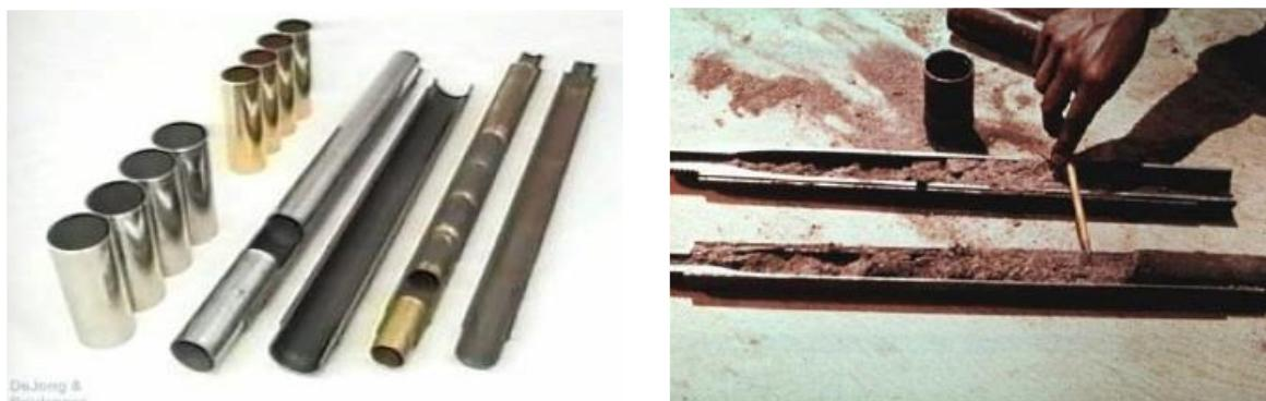
**Gambar 3-44 Tabung Penginti (*Split Spoon Sampler Barrel*)**
